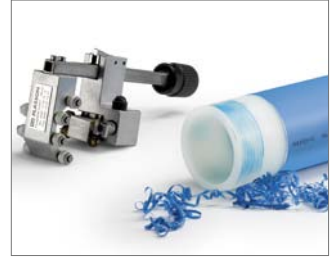
Fig. 68 When using a rotary scraper, peel off only a single layer. Provided that the outer layer (oxidation layer) has been removed, any residual pipe sheathing will not interfere with the welding process.
