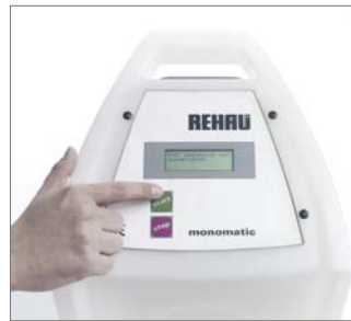
Fig. 101 Press the welding unit's start button and check the instructions as follows. Compare the welding parameters on the display with the values on the FUSAPEX electrofusion fitting.
