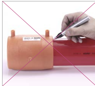
Fig. 118 Do not use the FUSAPEX electrofusion fitting as a marking aid.
