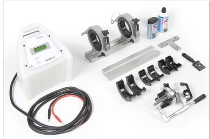
Fig. 85 Tools for creating joints
