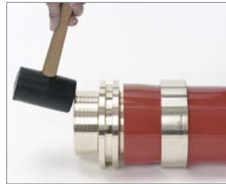
Fig. 31 6. The space between the fitting collar and the pipe end must be uniform on all sides. If necessary, use a rubber hammer to correct the position immediately after insertion.
