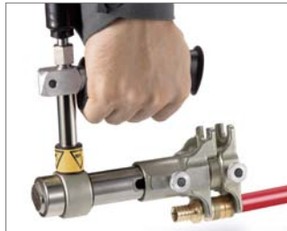
Fig. 16 6. Push the compression sleeve all the way up to the fitting collar. Once completed, pressure and temperature can be immediately applied to the joint.
