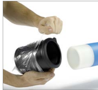
Fig. 44 6. Do not remove the electrofusion fitting from its bag until just before you intend to begin welding. If necessary, clean the fitting with Tangit.
