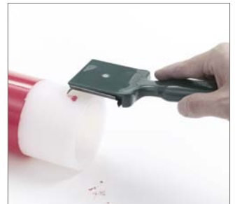
Fig. 94 All residual color must be removed with a manual scraper.
