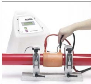
Fig. 100 Connect the REHAU welding unit; red cable to the red contact. The welding parameters are automatically detected.
