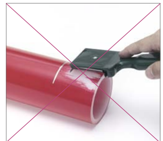
Fig. 124 Do not employ a manual scraper to scrape the pipe. This should only be used for subsequent scraping. Always employ a rotary scraper (refer to the price list).
