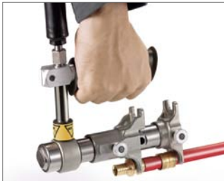
Fig. 15 5. Align the tool with the fitting and sleeve properly. Ensure the tool is sitting at a right angle to the joint. The compression jaws must be in full contact with the sleeve and fitting and be at a right angle to the connection.
