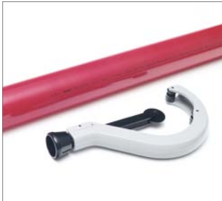
Fig. 89 Trim the pipe to the desired length. The cut face must be straight with respect to the pipe axis and must be smooth.
