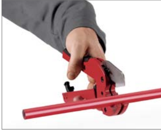
Fig. 11 1. Using a pipe cutter, cut the pipe to the desired length, burr-free and at a right angle.
