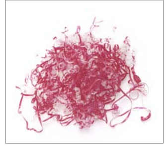
Fig. 112 Scraping should produce a long chip with a uniform thickness (0.1 to 0.2 mm); if required, replace the rotary scraper or knife.
