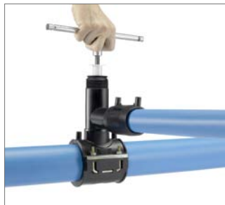
Fig. 61 9. At the conclusion of the pressure test, use an NW 12 Allen key to screw the hollow punch into the main pipe.
