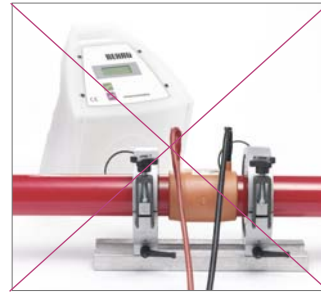
Fig. 127 During welding, the welding unit's connecting cable must not exert any force on the fitting.
