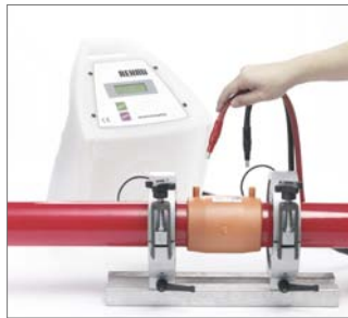
Fig. 104 An acoustic signal sounds once the welding process has been completed. The display reads "OK". The connections can now be removed.
