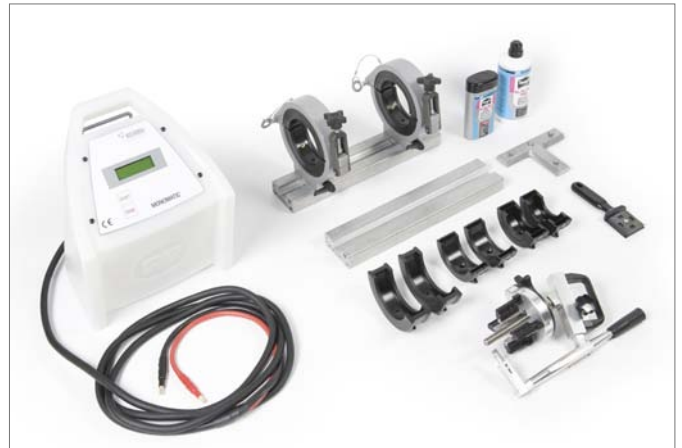
Fig. 38 Tools for creating joints
