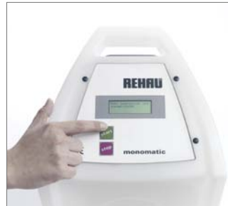
Fig. 58 6. Press the welding unit's start button and follow the instructions. Compare the welding parameters on the display with the values on the tapping clamp.
