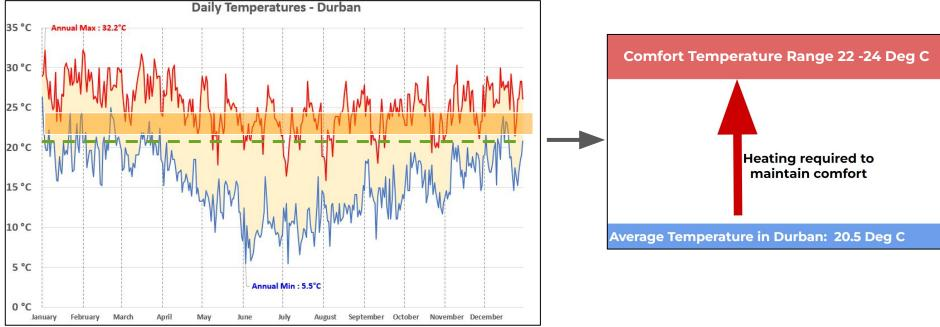
The temperature data along with known high humidity means this region would require some level of artificial cooling during day time, particularly in offices. Active heating is unlikely to be required within the office type areas. Controlling solar gains, reducing heat loss from the building will increase net-zero hours significantly.
