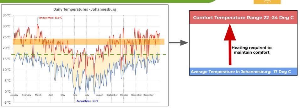
The climate summary shows that for the bulk of the year cooling is not required provided that solar gains are controlled. The average annual temperature across the year is significantly lower than the target comfort temperature. This indicates that active heating is required to maintain comfort during night time hours in particular. Controlling solar gains, reducing heat loss from the building will increase net-zero hours significantly.
