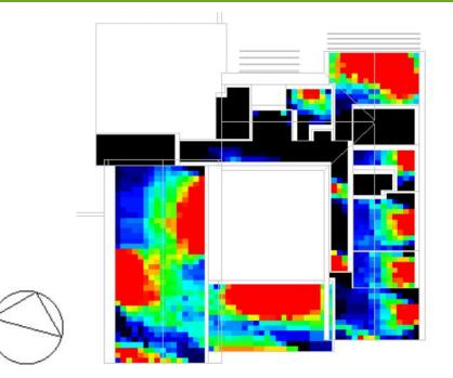
The annual sunlight exposure (aSE) metric identifies the percentage of the floor area that receives intense daylight, exceeding 1000 lux, for more than 250 work hours every year. a project must have a maximum aSE value of 10 percent. There are high levels of sunlight exposure on perimeter zones, with high levels seen in the main bedroom and covered patio zones. This indicates that these zones may have issues with glare.
