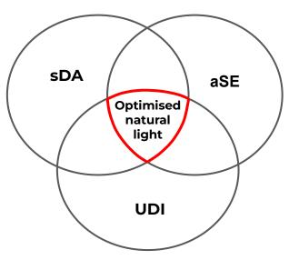
The annual sunlight exposure (aSE) metric identifies the percentage of the floor area that receives intense daylight, exceeding 1000 lux, for more than 250 work hours every year.
