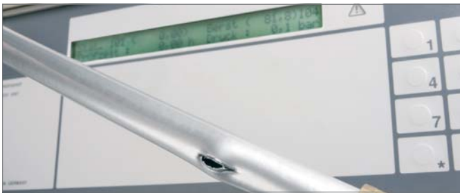
Fig. 3-1 Results of a burst pressure test with the universal pipe RAUTITAN flex
