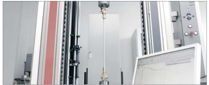
Fig. 3-3 Procedure of a tension test
